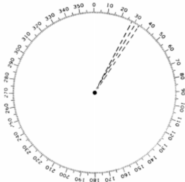
Figure 1308c. Ramark signal appearing as a broken radial line.
