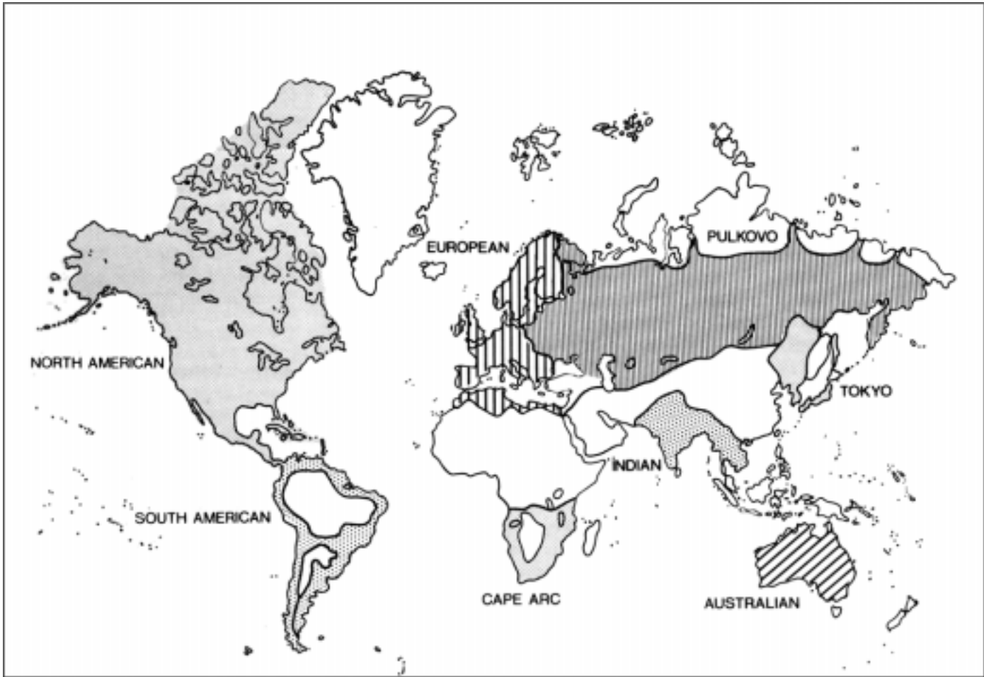
Figure 208. Major geodetic datum blocks.
