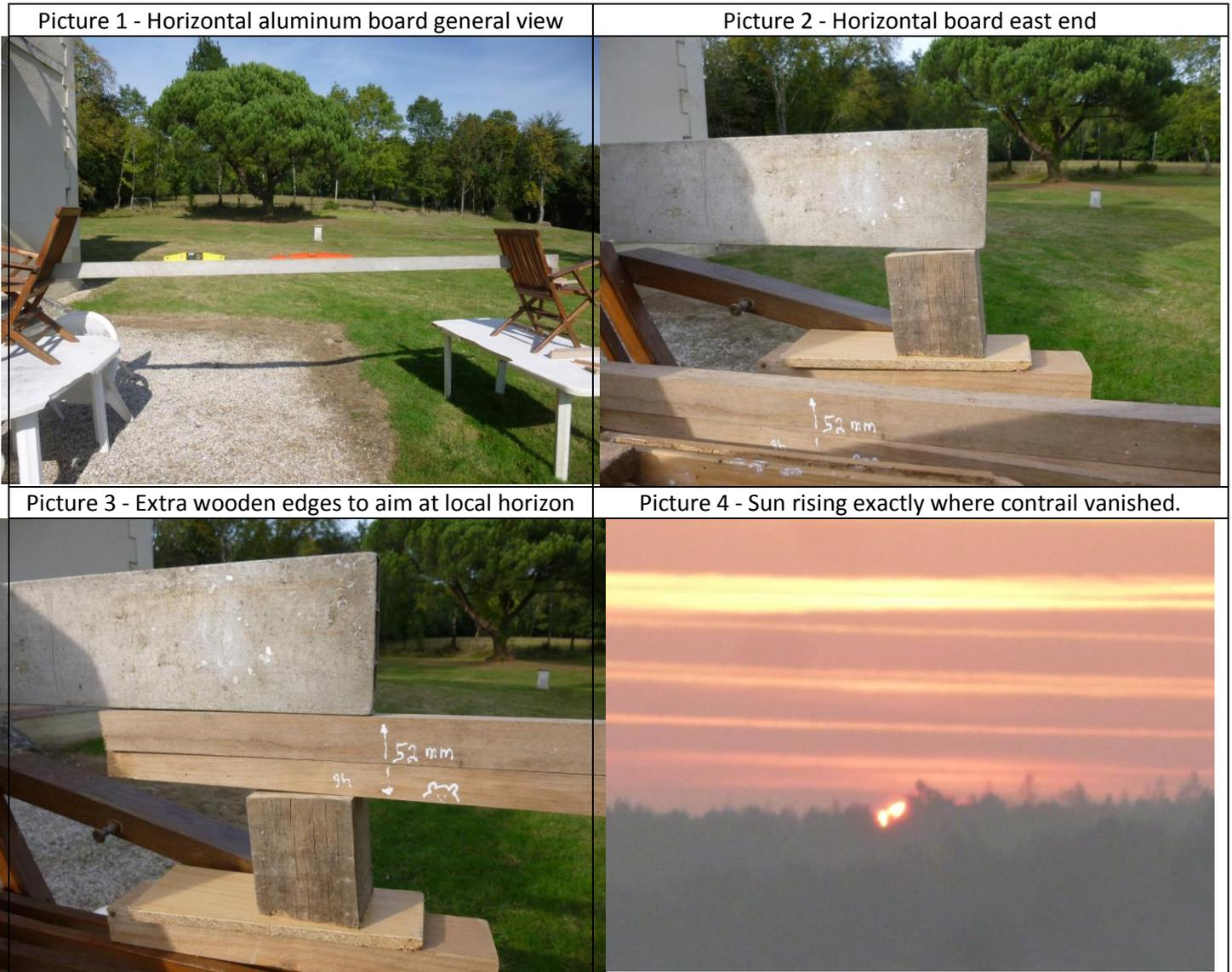
Picture 1 : One aluminum board: length 3,825 mm. To keep it rigid and to prevent it from falling flat with the wind maintain it “vertically” on its edge through the vertical rods of the backs of 2 garden chairs. Then horizontally level it with 2 “bubble levels” through inserting wooden wedges beneath it. Distance between both supports: 3,820 mm.
