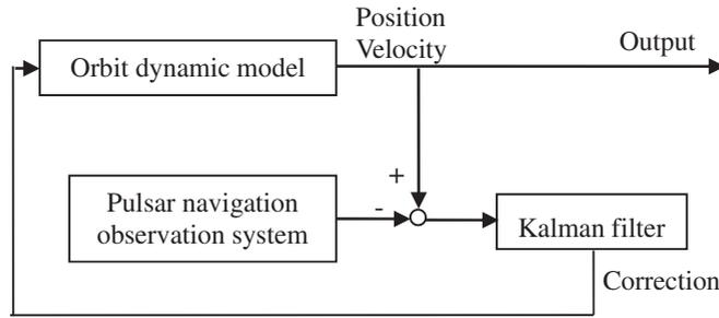
Figure 2. Principle of closed-loop correction.
