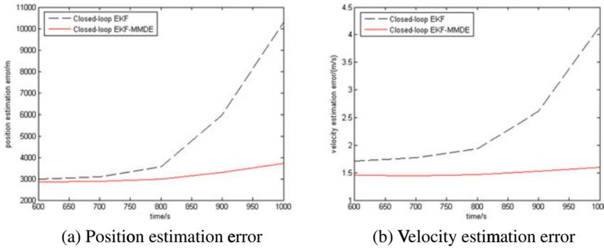
Figure 5. Estimation error with different observation period.
