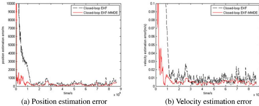
Figure 6. Estimation error of the two navigation methods.
