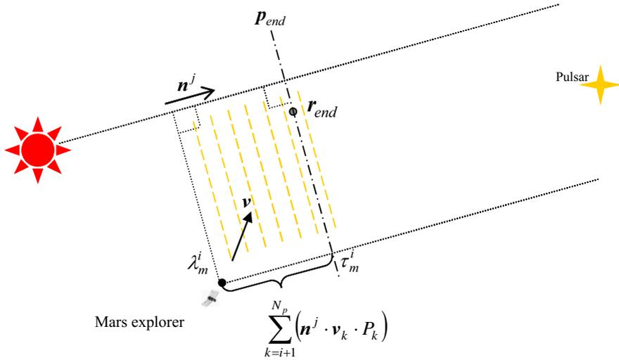
Figure 1. X-ray pulsar signal Doppler compensation.
