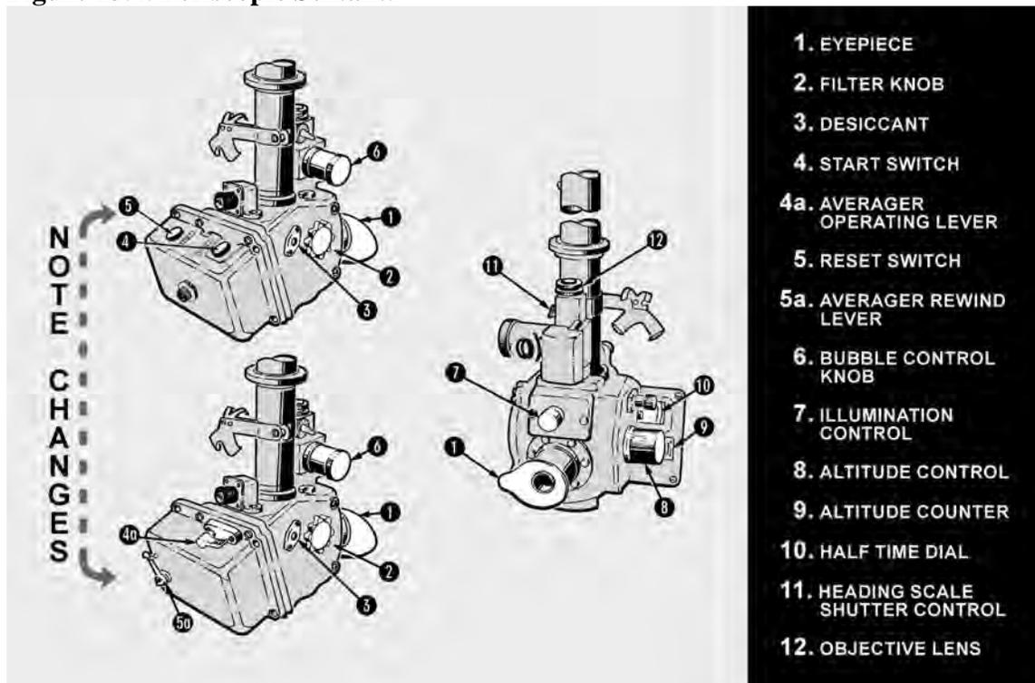
13.4.5. An eyepiece (1) rotates to correct the eyesight of the individual observer. Filters (2) are provided for selective use in the optical system so that the intensity of the sun's light might be adequately reduced. The filter control (2) is located on the left of the sextant.
