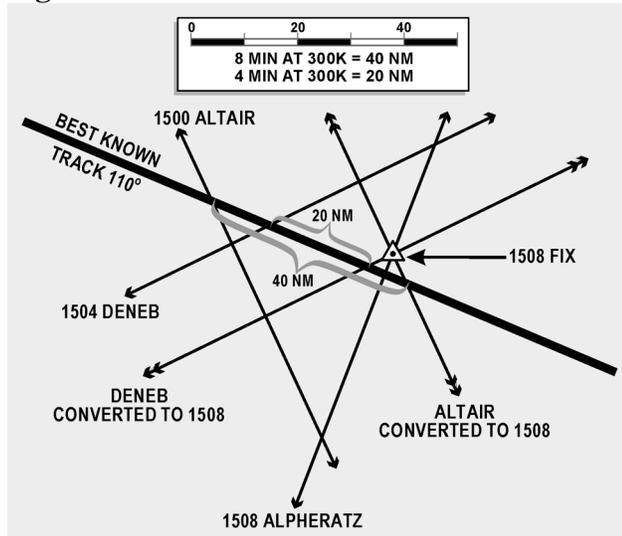
11.12.1. If, at any time, the LOP has to be retarded (moved back) to the time of the fix, use the following procedures. Using the reciprocal track and GS, obtain the correction in the regular manner for the number of minutes of difference. For example, suppose the fix is at 1800 and the last shot is at 1802.
