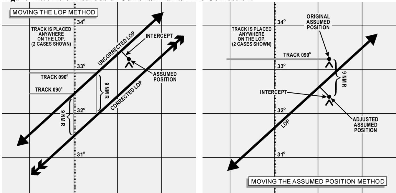
11.9.1. Notice that, in both methods, the corrected LOP is in the same place with respect to the original assumed position and that the intercept value is the same. The resultant LOP is the same regardless of the method used.
